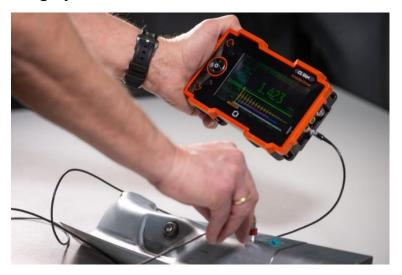
CL Go+ features a 5" crisp and clear display for advanced indoor and outdoor visibility, with large readouts to eliminate eye strain.
